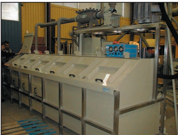
Ultrasonic cleaning unit for 14 parallel wires
